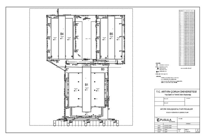
Picture 17 B blok rainwater drainage dateails
