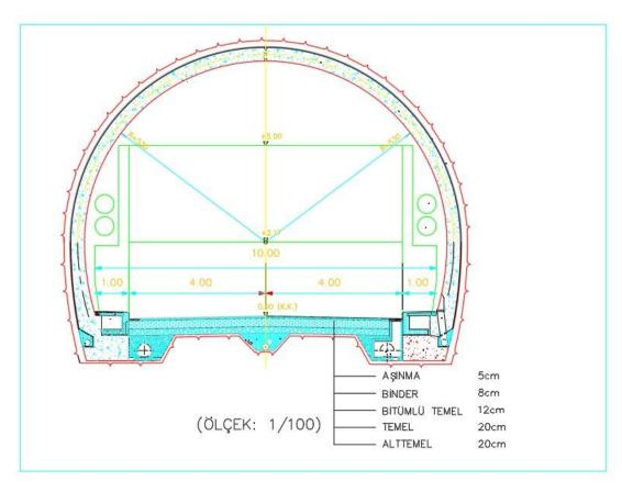
Picture 27 Trabzon Gündoğdu Project tunnel section
